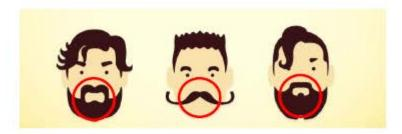
Edges of respirator create seal against clean-shaven skin. This moustache **does not** interfere with the respirator seal.
